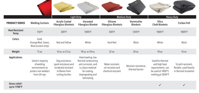
**NOTE:** Temperatures and applications are intended as a guideline only and not a guarantee of performance. SureWerx recommends the use of welding blankets in multiple layers to attain proper molten metal and radiant heat protection. It is the user's responsibility to monitor the activity and use of blankets/high-heat materials at all times. The user must inspect the blankets before use. Abnormal wear and tear should be removed from service.
