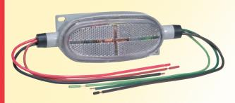
Betts circuit saver protects flasher circuits when extra lamp loads are used. It also extends switch life. Lamp loads of up to (24) 32 c.p. bulbs or 60 amps for both 4 and 7 wire 12 volt systems can be handled. Contains high quality Palladium relay contacts and has positive or negative ground. The Valox housing uses a clear 920143 shallow polycarbonate lens and is prewired with 12" pigtails. Mounting gasket, screws and wiring diagram are included. Surface mount.
