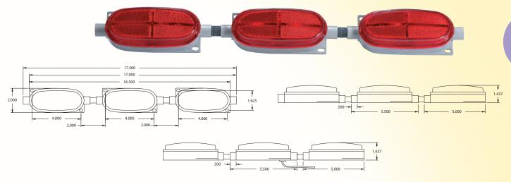
Features (3) REFLEX 920058 red or 920059 amber lenses and a tough valox body. Incandescent bulb version has a bulb replaceable shock mount socket and brass inserts with machine screws for a positive connection and uses (3) 168 bulbs. Surface mount.
