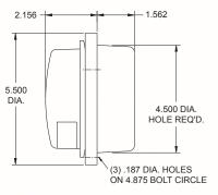
A compact size lamp available in both incandescent or LED. Lamp bodies are molded in a durable gray valox material. The incandescent bulb version features a 920141 red lens and uses a 920459 shock mount socket and 1157 bulb. The LED version is only available in valox and uses a 710025 Multi-voltage single LED lens assembly.
