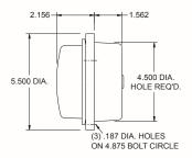
Halogen beacons may be used in place of strobes for many applications. Halogen beacons feature a tough valox housing and polycarbonate deep lens. Simplified circuitry along with good shock resistance insures less maintenance. The Halogen bulb is field replaceable. Mounting gasket, screws and 8" pigtails included.
