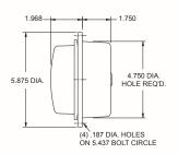
Halogen beacons may be used in place of strobes for many applications. Halogen beacons feature a tough valox housing and polycarbonate deep lens. Simplified circuitry along with good shock resistance insures less maintenance. The Halogen bulb is field replaceable. Mounting gasket, screws and 8" pigtails included.
