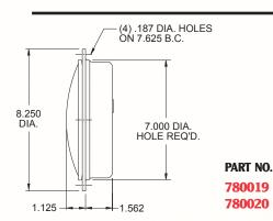
7" school bus lamp features polycarbonate shallow arrow lens and black valox body. Uses single contact shockmount bulb socket 920460 with single contact bulb 1156 and 920156 red or 920157 amber arrow lens. Has a 920420 choke seal with 18" abrasion resistant lead wire installed in rear. Mounting gasket and screws included. Recess mount.
