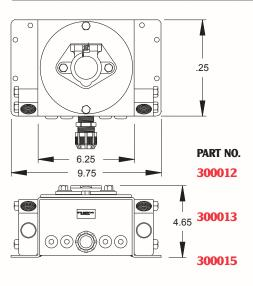
These new Betts heavy-duty nose boxes come completely sealed ready for installation. The 7-way socket comes with or without circuit breakers and is prewired to a 7-pole terminal disc. Machined glad hand (side blocks) 920042 are standard and replaceable. Fits existing trailer mounting brackets.
