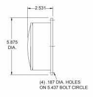
A surface mount lamp available in both incandescent and LED versions. Lamps will use either a 920134 red or 920135 amber shallow lens with a 920460 single contact socket, and 1156 bulb or a 710001 red or 710002 amber LED lens assembly.
