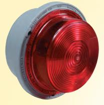
Strobe featuring high impact valox housing and polycarbonate lens. The Xenon flash tube with a life of 10 million flashes produces an (8) joule output per flash. Has a flash rate of 70 flashes per minute and an effective candle power of 102 with clear lens. Consumes 1 amp at 12 volts. Mounting gasket, screws and 8" pigtails included.
