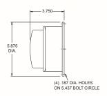
A dome or compartment lamp available in both incandescent and LED versions with a 920038 20 amp toggle switch. The incandescent version uses a 920140 clear deep lens, a 920460 socket and 1141 bulb. The LED version uses a 710027 single diode Multi-voltage LED clear lens assembly. All bodies must be provided with an internal ground.
