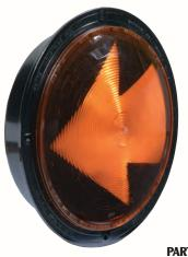
77 series lamps feature a valox body and are available in an incandescent or a LED version. The incandescent bulb version features a 920156 red arrow or a 920157 amber arrow lens and uses a 920460 socket and 1156 bulb. The LED version uses a 920687 red LED assembly for the red arrow or a 920688 amber LED assembly for the amber
