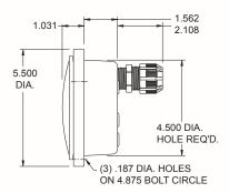
PART NO. 450061 Ready to install junction boxes with 7 pole terminal disc assembly. Features a durable Valox body and a polycarbonate shallow clear lens 920143. Boxes are drilled and tapped with entry fittings installed. Fittings include (1) cable entrance fitting 920402, (4) 1 hole cable choke seals 920413 and (1) 4 hole wire choke seal 920420. Mounting gasket and screws included. Recess mount.
