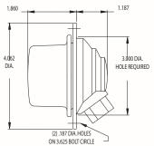
A special purpose lamp featuring a 920116 red or 920117 amber deep lens. Uses a double contact bulb socket 920126 and a 1157 bulb.
