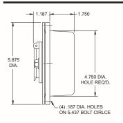
B40 series nose boxes are standard with heavy duty Valox bodies. Covers and bodies are sealed with Betts Snap-Seal O-rings. Mounting gasket and screws are included. Bodies must be drilled and tapped for wire entry. Recess mount.
