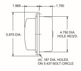
Strobe featuring high impact valox housing and polycarbonate lens. The Xenon flash tube with a life of 10 million flashes produces an (8) joule output per flash. Has a flash rate of 70 flashes per minute and an effective candle power of 102 with clear lens. Consumes 1 amp at 12 volts. Mounting gasket, screws and 8" pigtails included.
