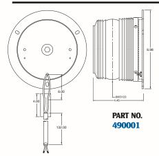
A high impact LED warning light with complete 360 degree display. Flash pattern can be changed with a button located on the base of the lamp. There are 4 flash patterns available.
