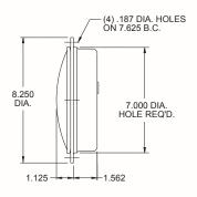
7" school bus lamp features polycarbonate shallow lens, black valox body and shock-mount bulb socket. Uses single contact bulb socket 920460 or double contact bulb socket 920459, single contact bulb 1156 or double contact bulb 1157, 920152 red, 920153 amber or 920151 clear lens. Has a 920420 choke seal with 18" abrasion resistant lead wire installed in rear. Mounting gasket and screws included. Recess mount.
