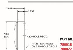
7" school bus lamp features polycarbonate shallow arrow lens and black valox flangeless body. Provided with internal mounting holes. Uses single contact shock-mount bulb socket 920460 with single contact bulb 1156, 920156 red or 920157 amber arrow lens. Has a 920420 choke seal with 18" abrasion resistant lead wire installed in rear. Mounting gasket and screws included. Surface mount.
