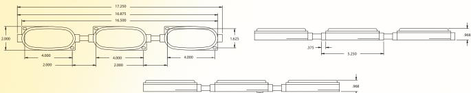
A low profile ID Bar lamp available in single contact incandescent bulb or LED version. The incandescent lamp features (3) 920049 red or 920050 amber lenses and uses (3) 67 bulbs.
