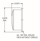
A dome or compartment lamp available in both incandescent and LED versions with a 920038 20 amp toggle switch. The incandescent version uses a 920133 clear shallow lens, a 920460 socket and 1141 bulb. The LED version uses a 710026 single diode Multi-voltage LED clear lens assembly. All bodies must be provided with an internal ground.
