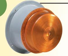
Strobe featuring high impact valox housing and polycarbonate lens. The Xenon flash tube with a life of 10 million flashes produces an (8) joule output per flash. Has a flash rate of 70 flashes per minute and an effective candle power of 102 with clear lens. Consumes 1 amp at 12 volts. Mounting gasket, screws and 8" pigtails included.
