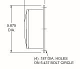
Junction boxes feature a polycarbonate shallow clear lens 920143. They are available with or without a 7 pole terminal disc with hardware. Boxes must be drilled and tapped unless otherwise stated. Mounting gasket and screws included. Recess or surface mount available.
