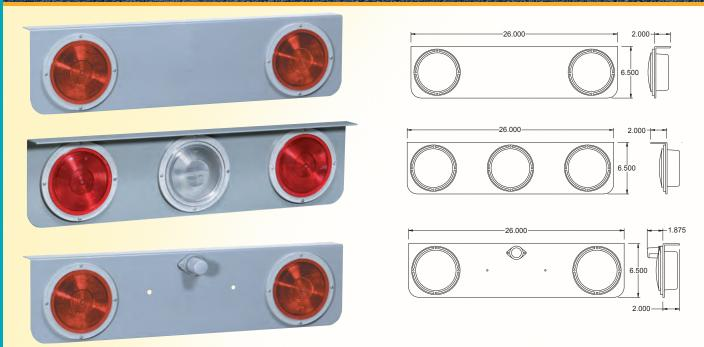
Betts rear tractor modules feature 12 gauge powder coated angle steel frames. Modules are available in incandescent bulb, multi-diode LED, and Multi-voltage single diode LED's. Units are completely sealed from module to cab and include 14 ft. of either 4 or 5 conductor cable.
