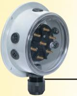
For use with non-piped conventional wiring. Ready to install junction box with a 7 pole terminal disc assembly. Provided with a polycarbonate shallow clear lens 920143. Models are drilled and tapped with entry fittings installed. Mounting gasket and screws included. Surface mount.
