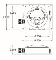
This is a heavy duty aluminum junction box with 16 brass circuit studs. It is completely sealed and has 12 wire entrances distributed on 4 sides. The clear Snap-Seal polycarbonate cover enables easy access for circuit checking. Sealed entries include (1) cable entrance fitting 920402, (1) 1/2" N.P.T. plastic plug, (10) one hole cable choke seals 920413. A 16 pole hardware package is included. Surface mount.
