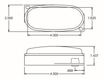
Incandescent lamp version features a REFLEX 920058 red or 920059 amber lens. The lamp features a bulb replaceable shock mount socket and brass inserts with machine screws for positive connections and uses a 168 single contact bulb.
