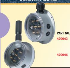
Ready to install junction boxes which each feature a 7 pole terminal disc assembly. Features a heavy duty Valox body and a polycarbonate shallow clear lens 920143. Boxes are drilled and tapped with entry fittings installed. Mounting gasket and screws included. Surface mount.
