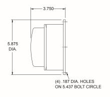
A surface mount lamp available in both incandescent and LED versions. The incandescent version features a 920144 red or a 920145 amber deep lens and uses a 920460 single contact socket and a 1156 bulb or a 920459 double contact socket and a 1157 bulb. The LED version uses a 710011 red or a 710012 amber LED lens assembly.
