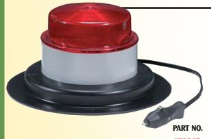
Strobe featuring high impact valox housing and polycarbonate lens. The Xenon flash tube with a life of 10 million flashes produces an (8) joule output per flash. Has a flash rate of 70 flashes per minute and an effective candle power of 102 with clear lens. Consumes 1 amp at 12 volts. Includes suction gasket, magnet, 8' of wire and cigarette lighter adapter.
