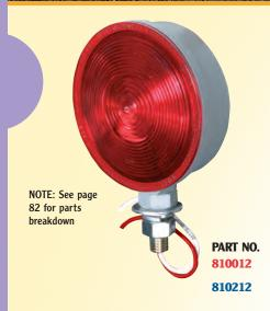
Pedestal mount aluminum body lamp is available in an incandescent and LED version. Incandescent bulb version features a 920134 red or 920135 amber lens. The single contact bulb version uses a 920015 single contact socket and 1156 bulb and the double contact lamp uses a 920013 double contact socket and 1157 bulb. The LED versions use a 710003 red or 710004 amber LED lens assembly.
