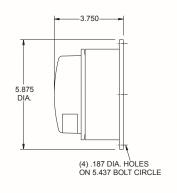
A tough valox body lamp available in an incandescent bulb or LED version. The incandescent bulb version features a 920141 red lens, a 920459 shock mount socket and an 1157 bulb. The LED version uses a 710025 Multi-voltage single diode lens assembly. Surface mount.
