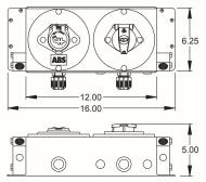
ABS heavy duty dual socket nose box ready for installation. Comes with ABS socket 920554 and standard socket 920427. Standard socket is prewired to a 7 pole terminal disc. A red and white jumper wire is wired from disc to disc to provide a ground and alternate ABS power source based on the trailer wiring.
