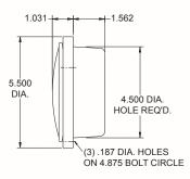
Back up lamps are available in incandescent and in both multi and single diode Multi-voltage. LED lamps are designed to operate for either 12 or 24 volt systems. Incandescent lamps use a 920139 lens with a 920460 socket and 1156 bulb. Multi-diode lamps use a 710037 LED clear lens assembly and the single diode lamp uses a 920139 lens with a 920691 single diode LED assembly.
