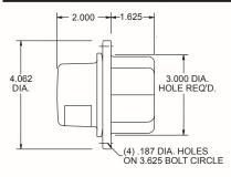
An incandescent lamp molded in durable gray valox. Features a 920113 red lens and a uses a 920104 shock mount socket and 67 bulb.
