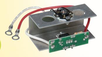
A high output Multi-voltage single LED assembly. Assemblies meet F.M.V.S.S. 108 compliance for stop/turn/tail or marker functions while operating within a voltage variance range from as little as 8 volts to as high as 44 volts without degrading the LED or circuitry. Assemblies all come as a double contact but can be wired internally to meet any functions needed.
