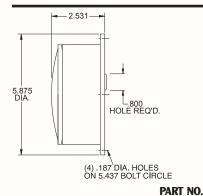
A tough durable black bodied valox light available in both incandescent bulb or LED versions. The incandescent bulb version features a 920134 red shallow lens with a 920459 double contact shock stopper socket and a 1157 bulb. The LED version features a 710001 double contact shallow red LED lens assembly. A 920420 wire choke seal is installed in the rear of the lamp with 18" abrasion resistant lead wires. Surface mount.
