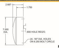
7" school bus lamp features polycarbonate shallow lens, black valox flangeless body and shock-mount bulb socket. Provided with internal mounting holes. Uses single contact bulb socket 920460 or double contact bulb socket 920459, single contact bulb 1156 or double contact bulb 1157, 920152 red, 920153 amber or 920151 clear lens. Has a 920420 choke seal with 18" abrasion resistant lead wire installed in rear. Mounting gasket and screws included. Surface mount.
