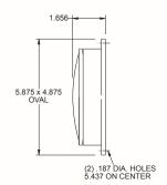
A meter or cabinet lamp that uses a shielded 920055 deep lens and a 67 incandescent bulb.
