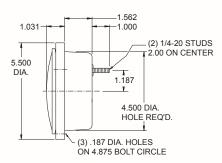
A tough durable black bodied valox light available in both incandescent bulb or LED versions. The incandescent bulb version features a 920134 red shallow lens with a 920459 double contact shock stopper socket and a 1157 bulb. The LED version features a 710001 double contact shallow red LED lens assembly. Stud mount provided with 1/4" x 20" mounting studs. Both lamps provided with a 920420 wire choke seal installed in the rear of the lamp with 18" abrasion resistant lead wires.
