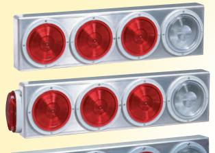
Four lamp modules, completely sealed with no external splices and provided with a 920420 wire choke seal so they are ready to install. Box frames are available in aluminum or powder coated mild steel with or without side marker. Modules consist of (3) red lamps wired as single or double contact, a back up lamp and a side marker option. Lamp bodies are 40 series valox and
