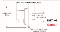
A self grounding valox body lamp that features a 920113 lens. Uses a 920127 socket and 67 bulb. Provided with a 1/4" N.P.T. rear entry. Surface mount.
