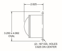
All 57 series lamps are molded from a durable valox material and must now be grounded internally by the use if an additional wire or by the use of a ground screw drilled thru the base of the lamp from the inside making ground contact using the socket or LED lens assembly ground wire and the metal mounting surface.
